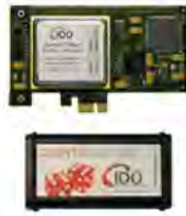
[Quantis, IDQuantique] - 4Mbps - PCIe, USB - photon dispersion
